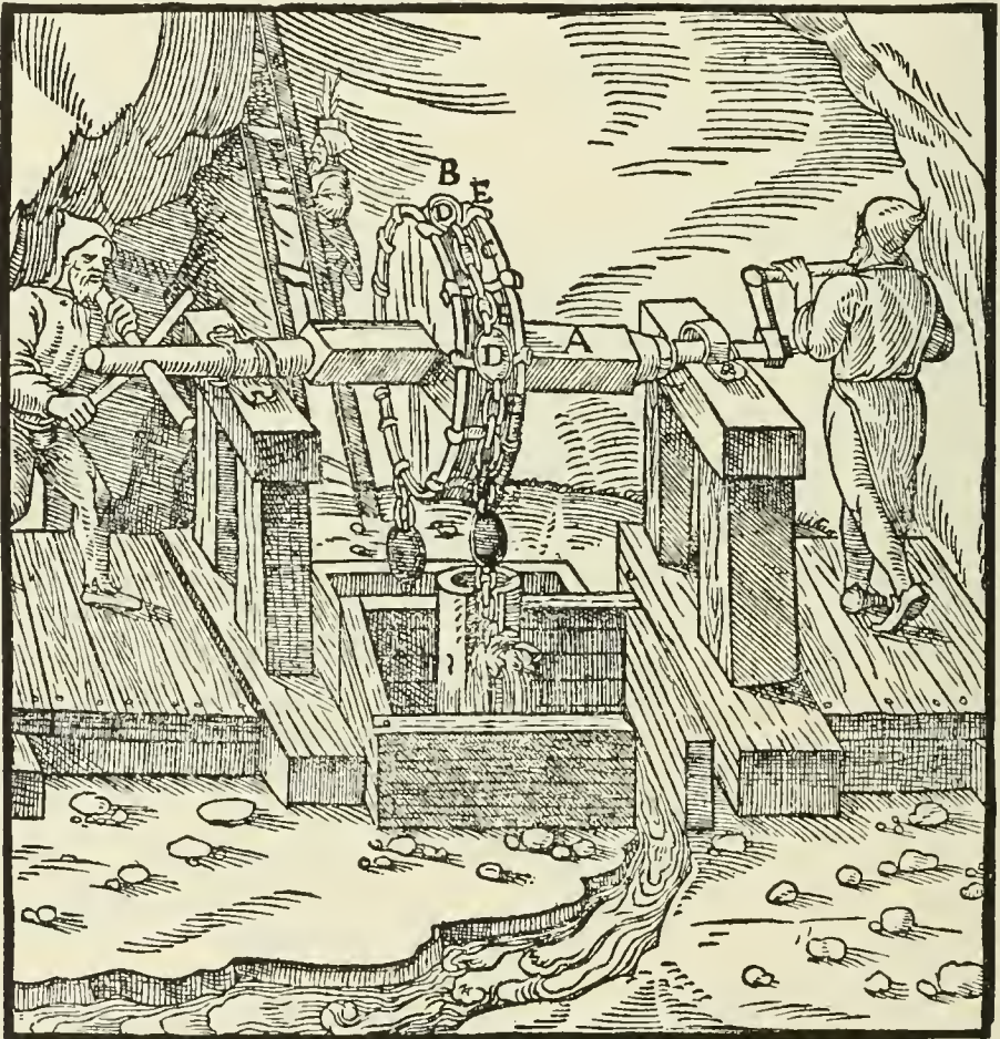
A—AXLE. B—DRUM. C—DRAWING-CHAIN. D—BALLS. E—CLAMPS.
